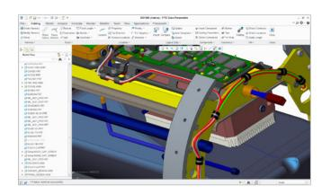
Automated cabling design capabilities make it easy to move components and connectors without manually rerouting wires and cables.
